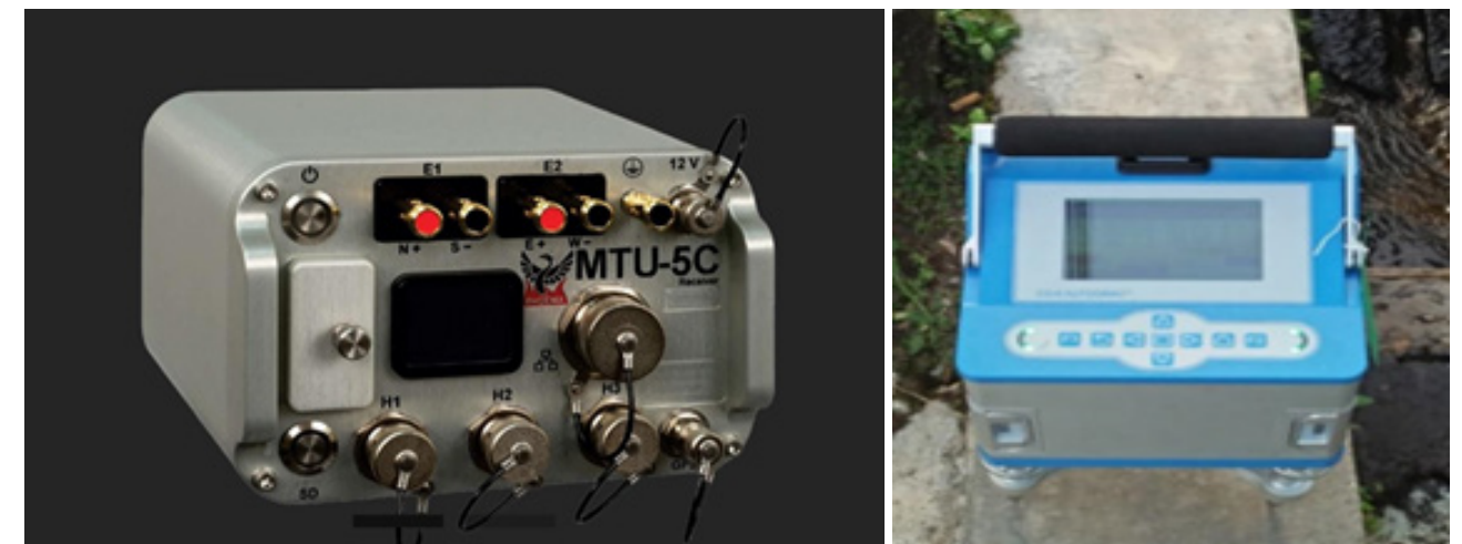
Magnetotelluric and gravimeter for geophysical survey
